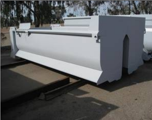
17' Semi Elliptical Steel Dump Bodies (51547)
